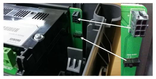
Figure 31. Battery On/Off Switch and Battery Connector
