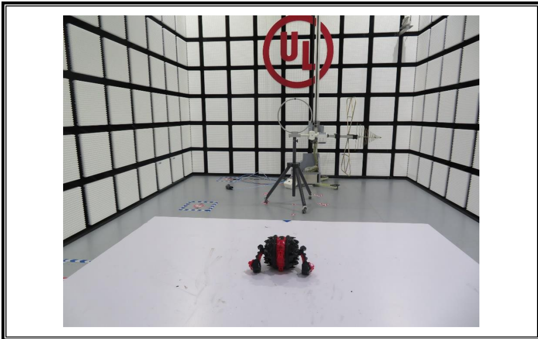
RADIATED RF MEASUREMENT SETUP (Below 30MHz)
