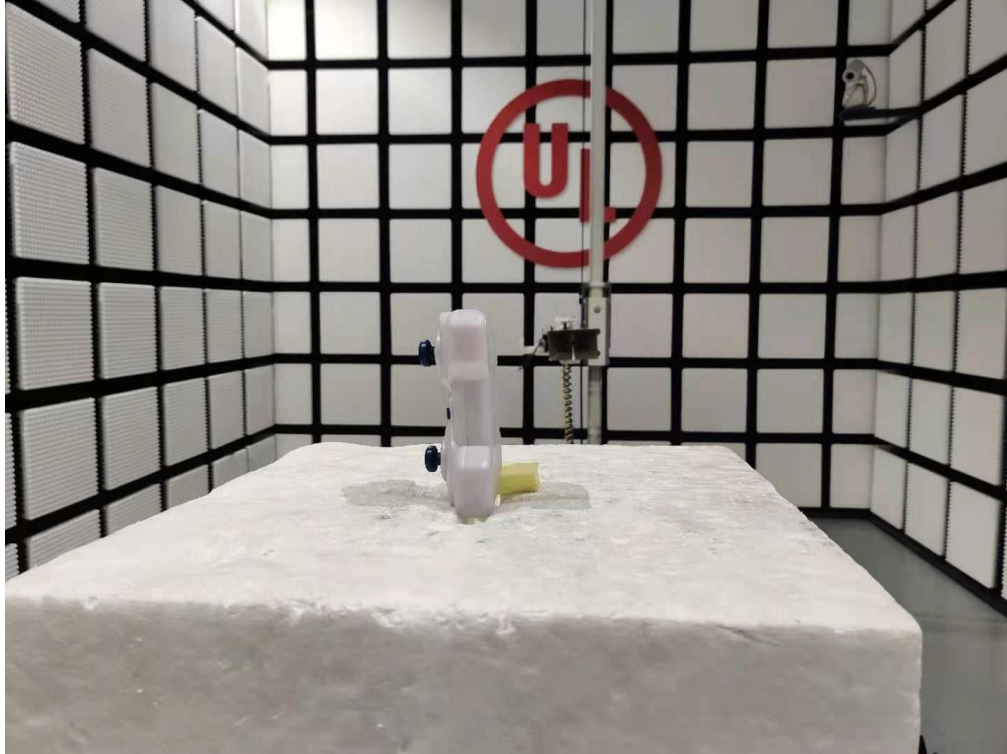
Radiated Disturbance Setup (Above 1 GHz – Z axis)
