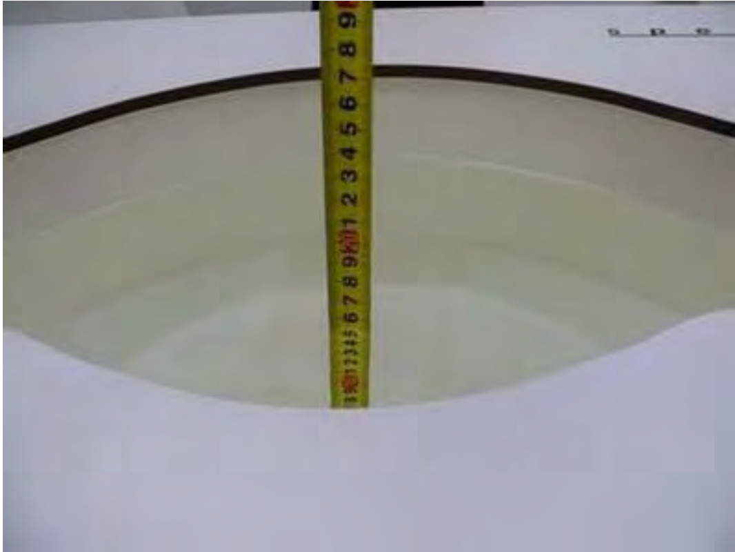
Picture 3: Liquid depth in the flat Phantom (2450 MHz, 15.3cm depth)
