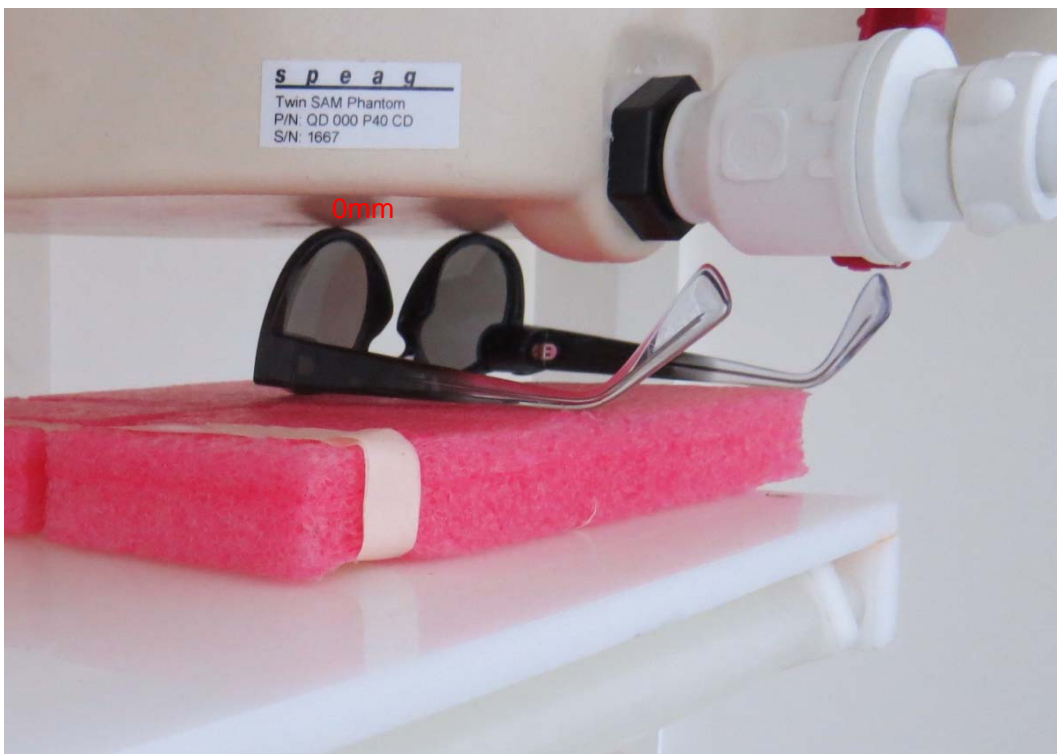
Picture 6: Bottom Side, the distance from EUT to the bottom of the Phantom is 0mm
