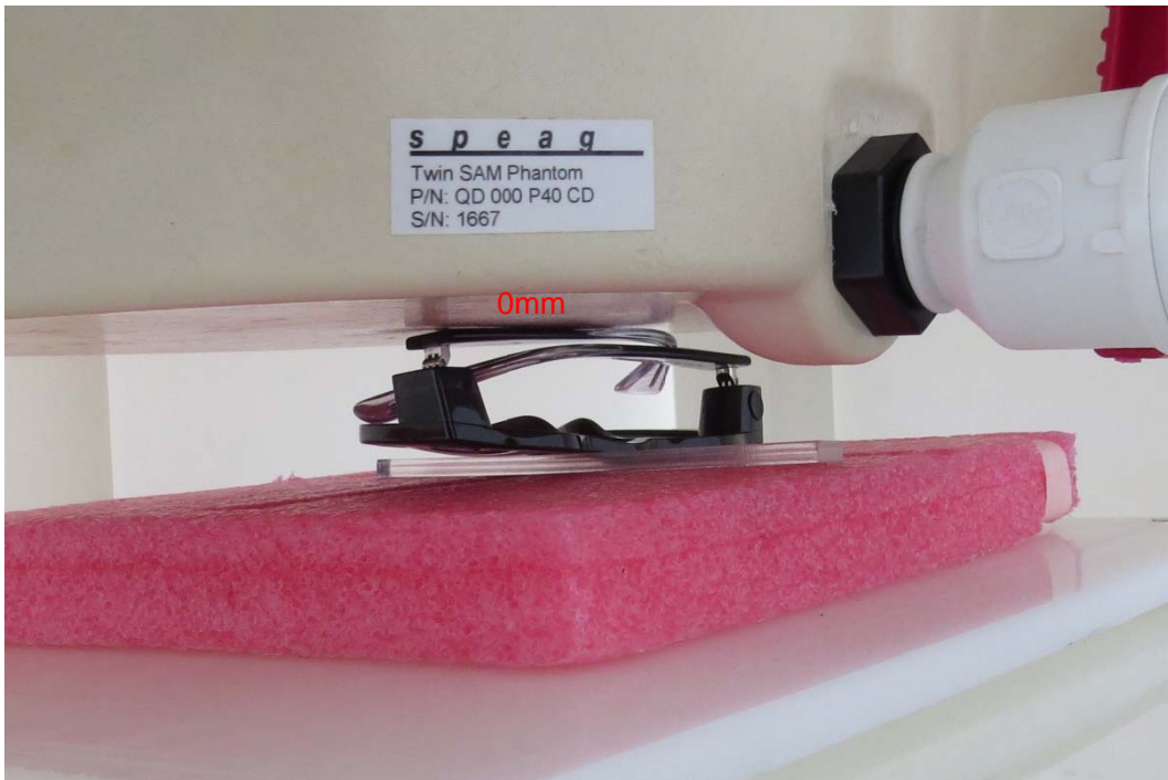
Picture 1: Back Side (Close), the distance from EUT to the bottom of the Phantom is 0mm
