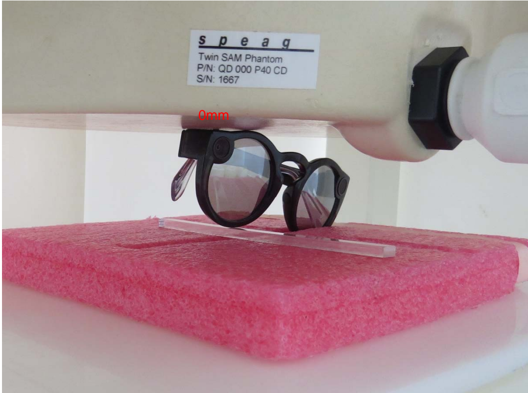
Picture 5: Top Side, the distance from EUT to the bottom of the Phantom is 0mm
