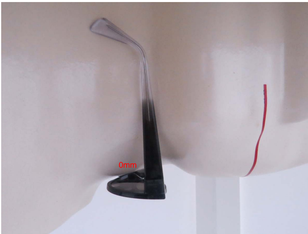
Picture 2: Back Side (Open Inside), the distance from EUT to the bottom of the Phantom is 0mm
