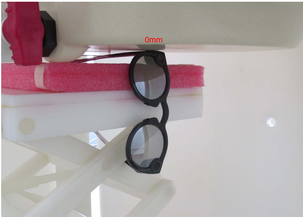
Picture 4: Right Side, the distance from EUT to the bottom of the Phantom is 0mm
