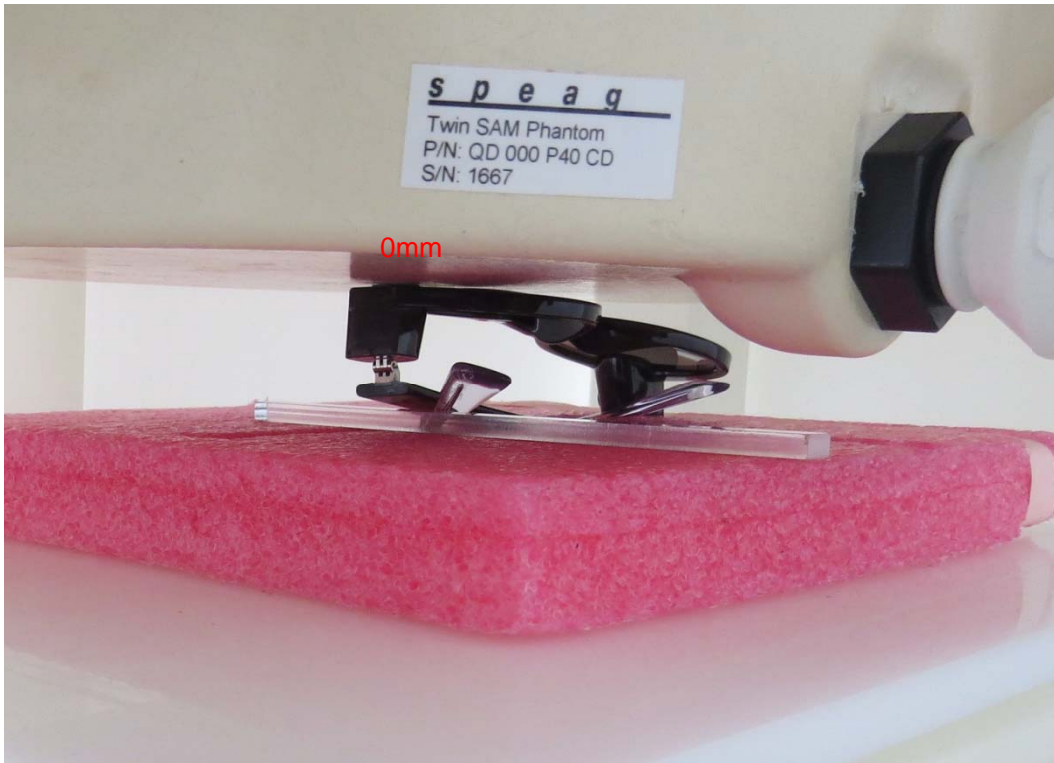
Picture 3: Front Side, the distance from EUT to the bottom of the Phantom is 0mm
