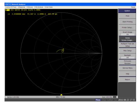
2450MHz Head calibrated impedance 55.713 $\Omega$ ; measured impedance: 55.167 $\Omega$  (within 5 $\Omega$ )
