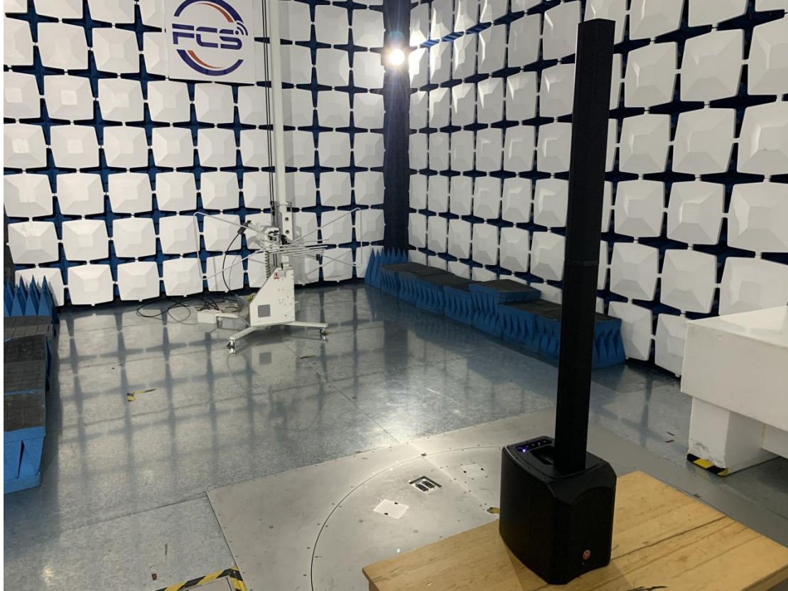
Above 1GHz for radiated emission test setup
