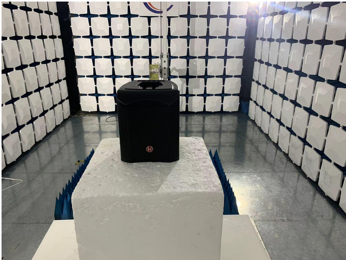
Above 1GHz for radiated emission test setup
