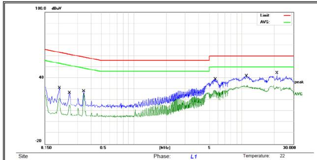
Limit:FCC Part 15B\_(0.15-30MHz) \_Main\_QP Power: AC 240V/50Hz Humidity: 51 %
