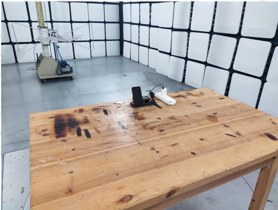
Photo of Radiation Emission Test
