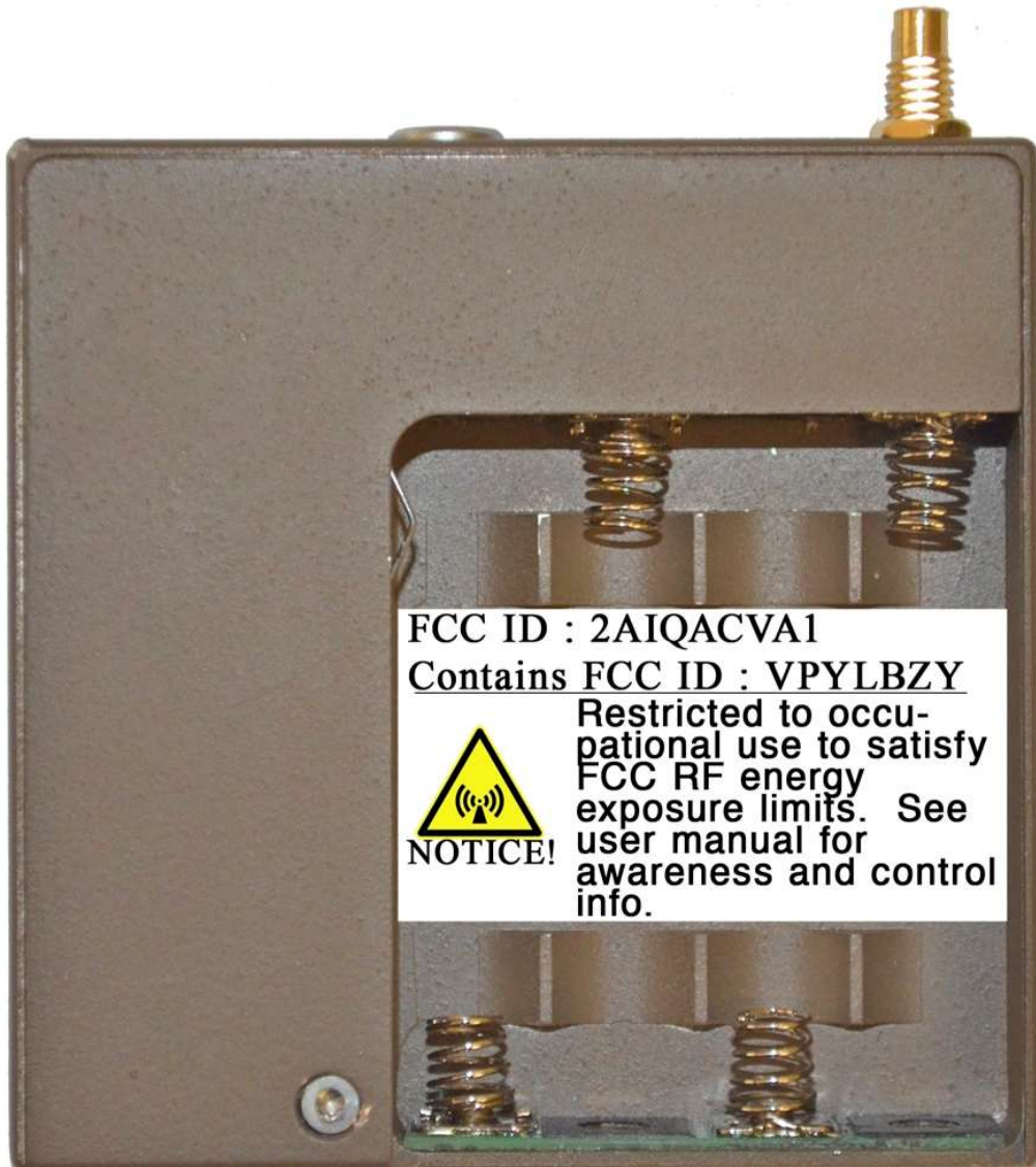
Proposed FCCID and RF Exposure warning label. Device to be shipped without batteries installed.
