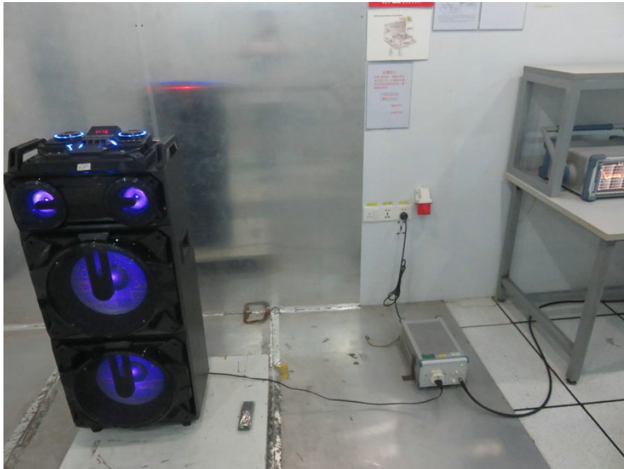
1 Photo of Power Line Conducted Emission Measurement
