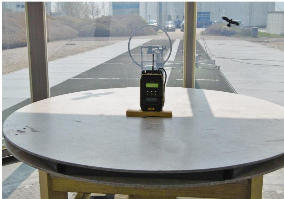
Test setup 30 MHz – 1000 MHz:
