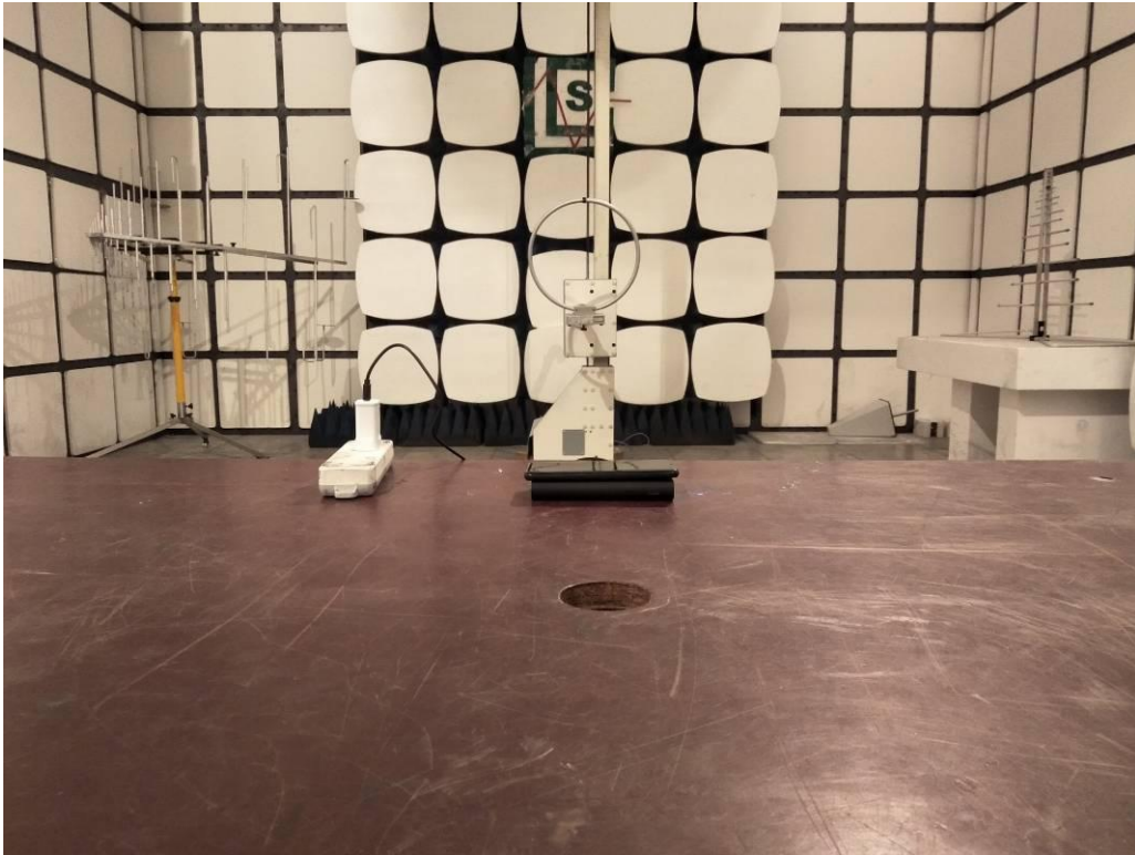
Radiated Emission below 30MHz-AC adapter charge mode
