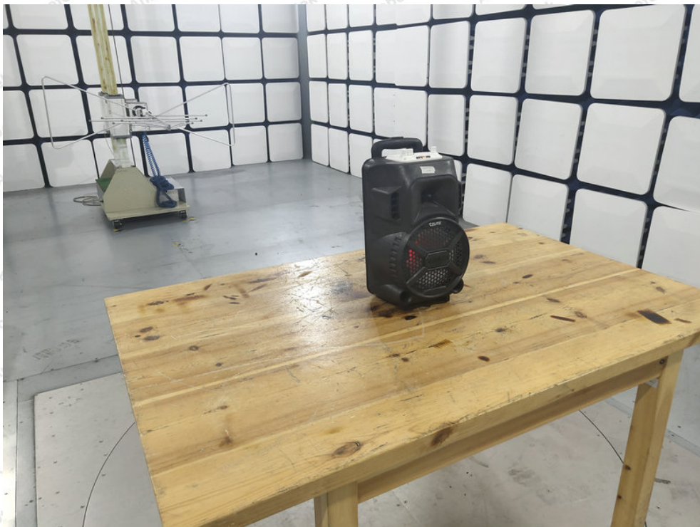
Photo of Radiation Emission Test
