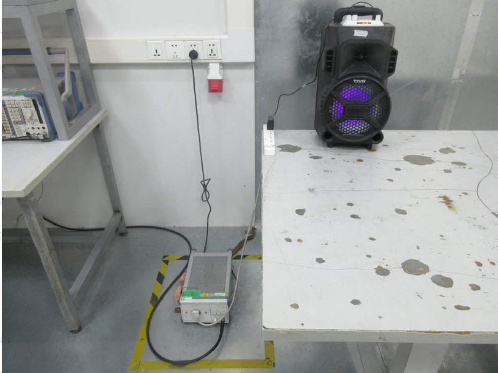
Photo of Power Line Conducted Emission Test
