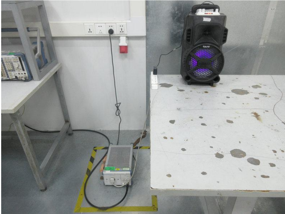
Photo of Power Line Conducted Emission Test
