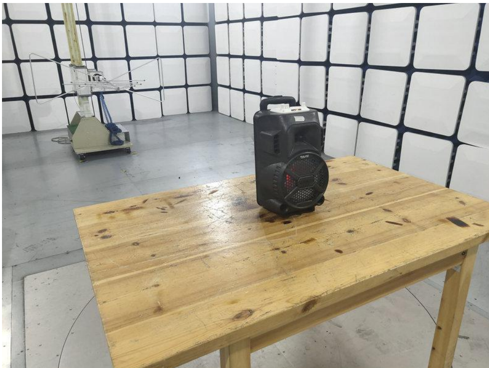
Photo of Radiation Emission Test
