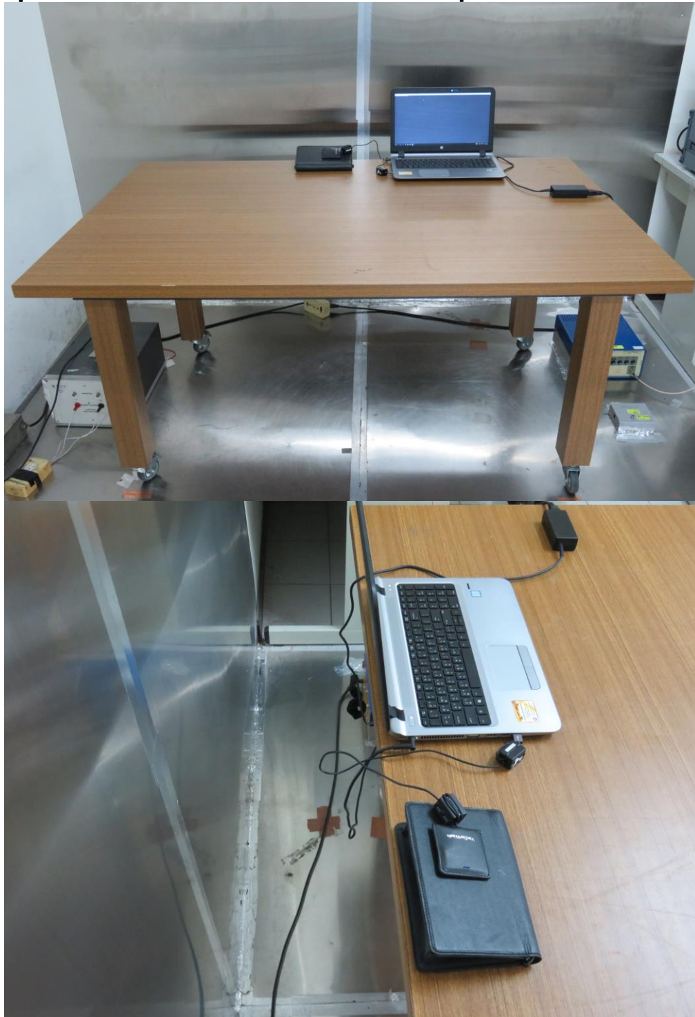
Photograph – Conducted Emission Test Setup
