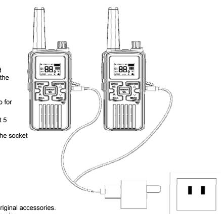
• Rotate the PWR/VOL control knob clockwise until a" ka-ka "sound is heard to turn on the power When you receive calls ,the knob provides you the ability to change the volume for your listening habits. When shutting down the transceeiver, you need to rotate it counterclockwise a "ka-ka" sound is heard.
