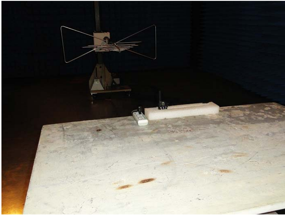
Radiated emission test view
