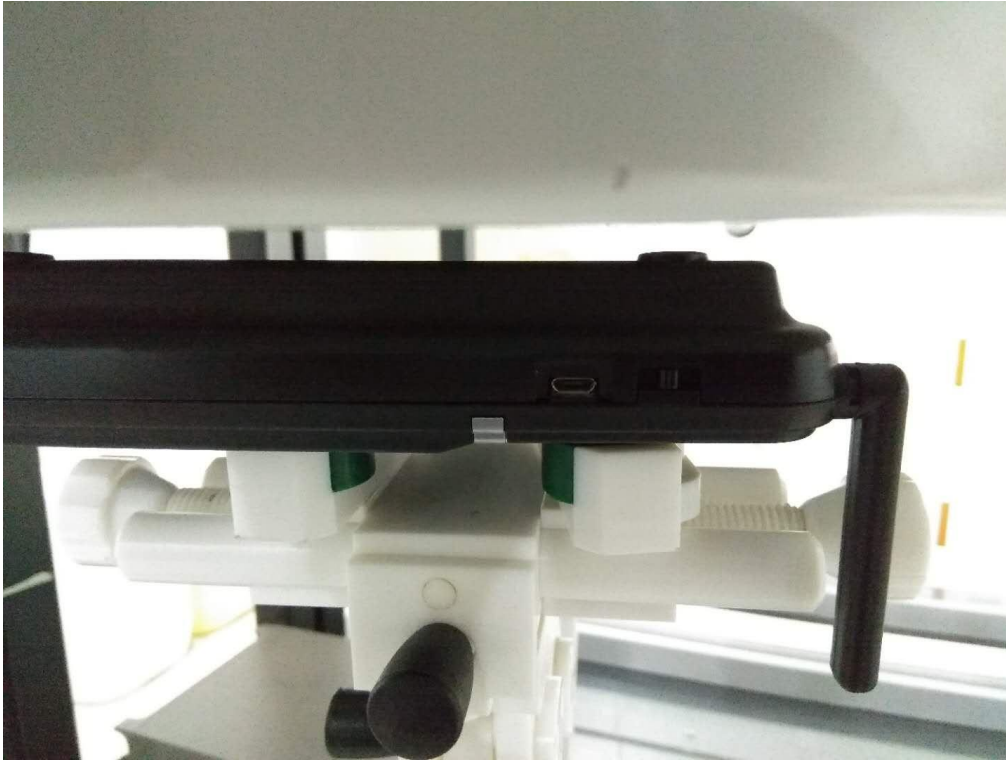
Body Back side(separation distance is 5mm)_the antennas at 90 degrees
