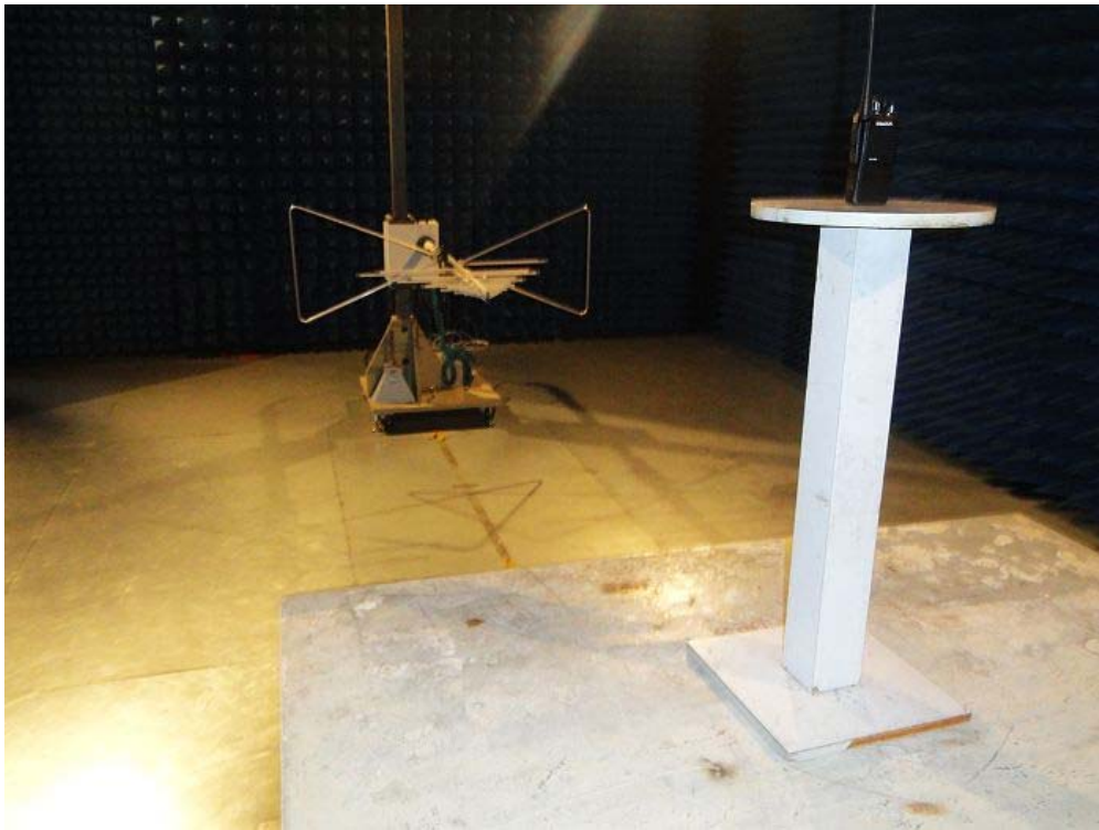
Spurious Radiated emission test view
