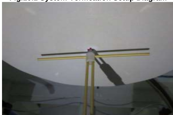
Fig.10.2 Photo of Dipole setup
