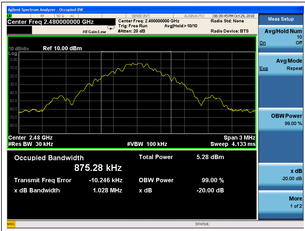
(GFSK, Channel 78, 2480MHz)
