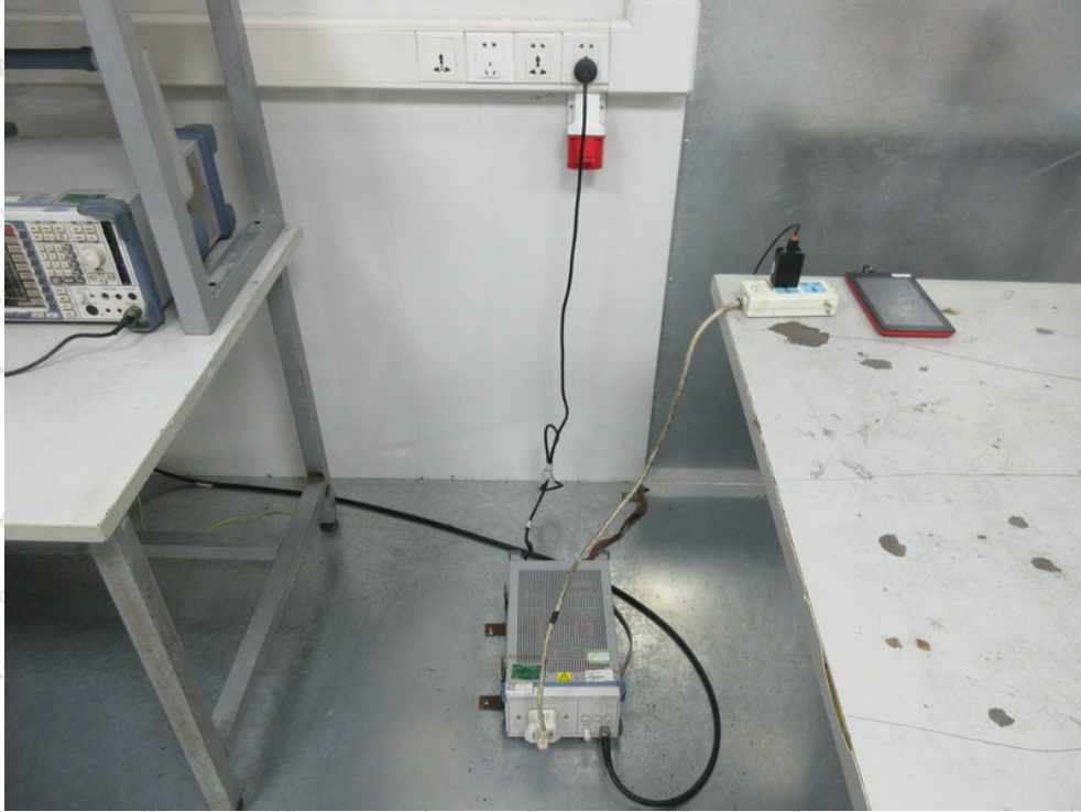
Photo of Conducted Emission Measurement
