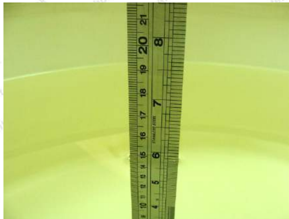
Photo of Liquid Height for Body SAR
