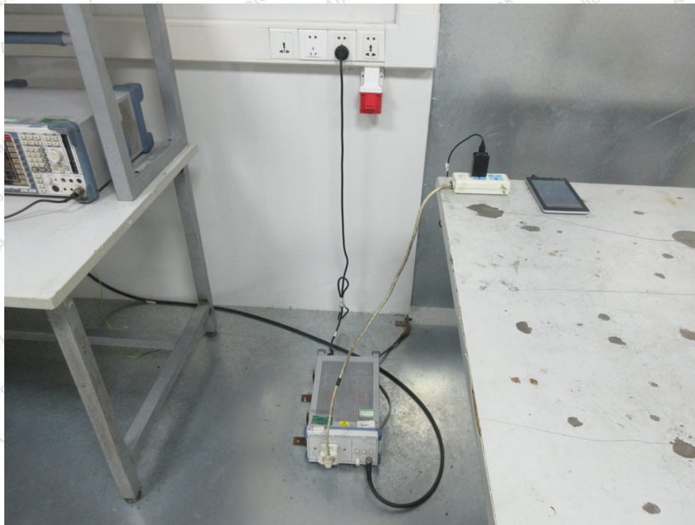
Photo of Conducted Emission Measurement
