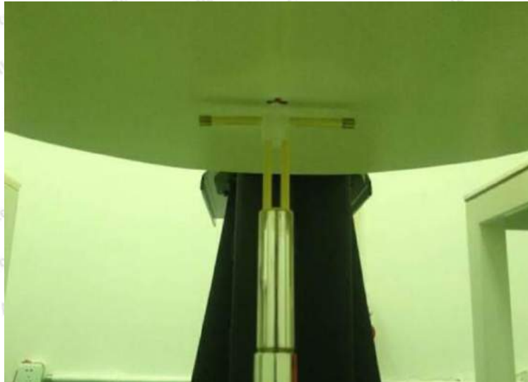
Photo of Dipole Setup
