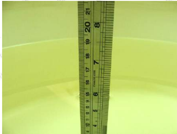
Photo of Liquid Height for Body SAR
