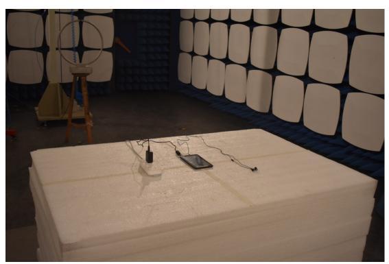
3. Radiated emission (9KHz-30MHz)
