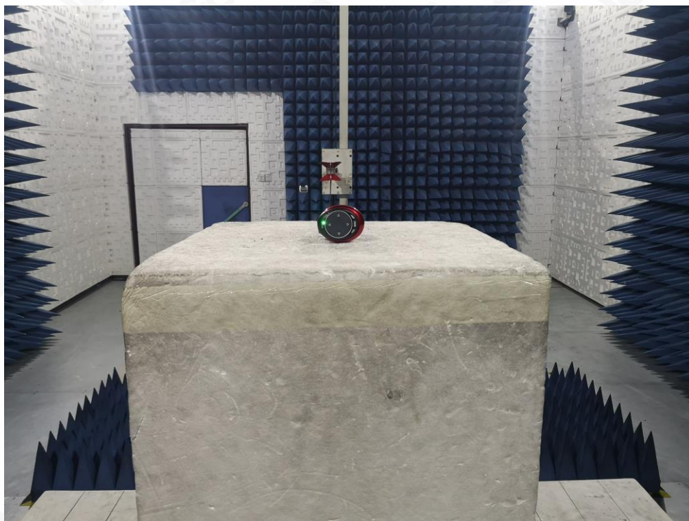
FCC RADIATED EMISSION TEST SETUP ABOVE 1GHZ
