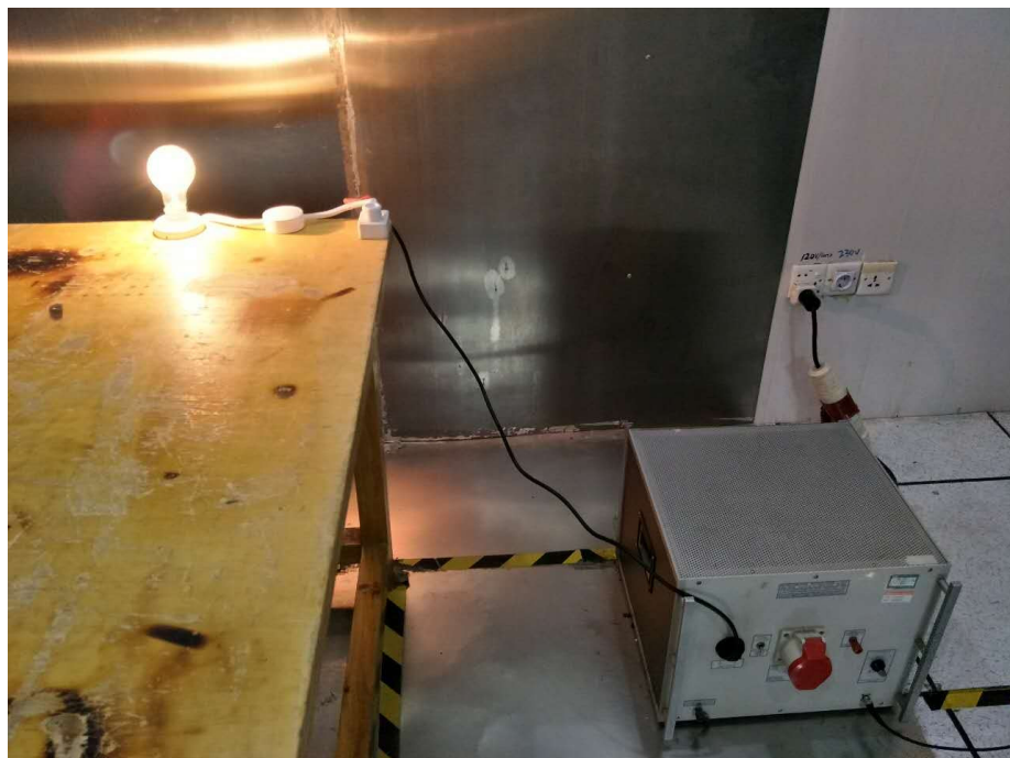
Photograph – Conducted Emission Test Setup
