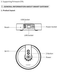
Smart gateway is a Z-WAVE controller with smart chips, it can format
