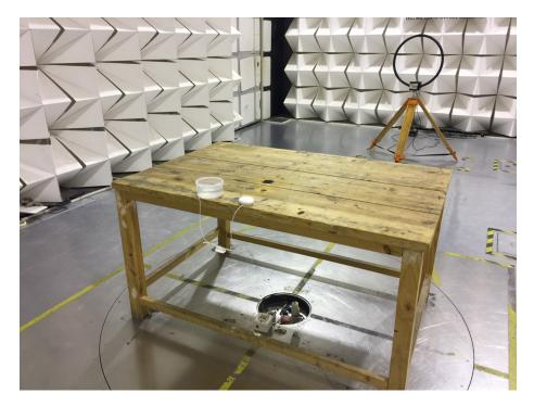
Test frequency from 30 MHz to 1 GHz at test
