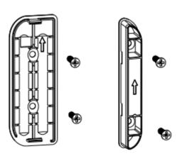
3) Attach the double-sided mounting tape to the covers and to adhere to the wall, door or window frame.
