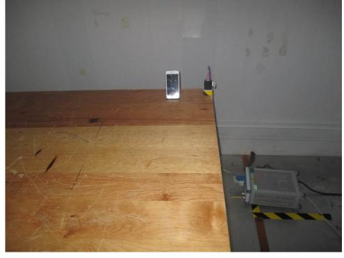
8.2 Radiated Emissions (30MHz-1GHz) Test Setup
