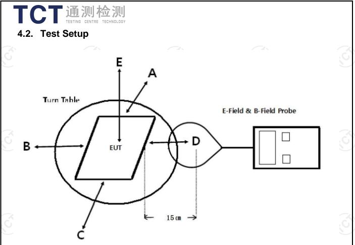
Note: Measurements should be made from all sides and the top of the primary/client pair, with the 10cm measured from the center of the probe(s) to the edge of the device.
