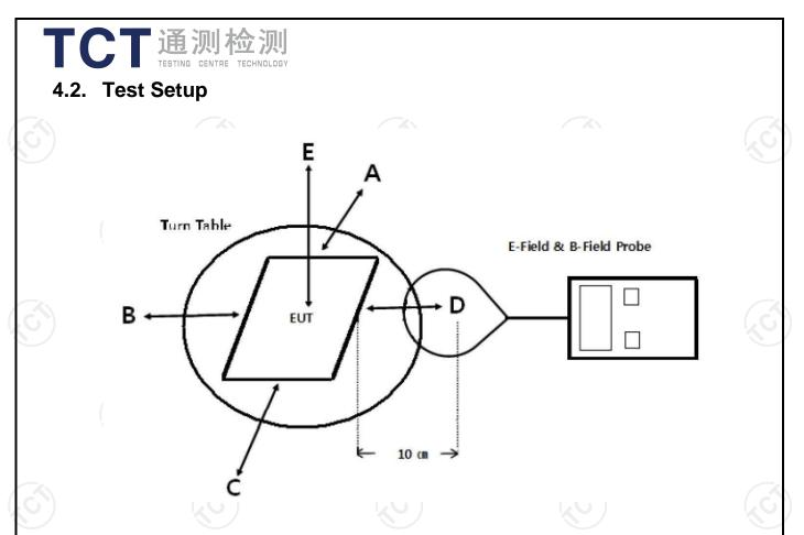
Note: Measurements should be made from all sides and the top of the primary/client pair, with the 10cm measured from the center of the probe(s) to the edge of the device.
