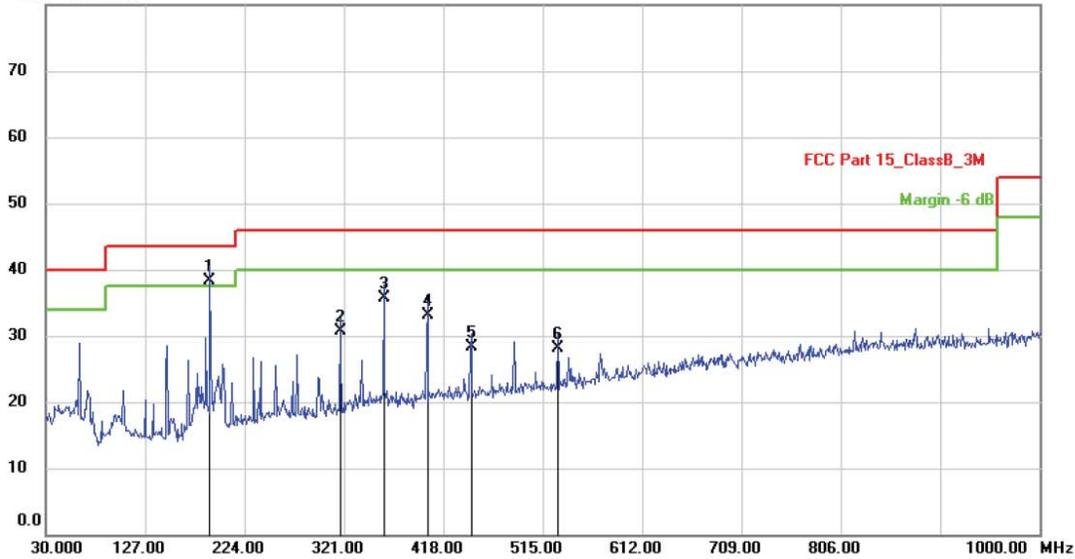
Site: 3m Chamber      Polarization: *Vertical*      Temperature: 26
