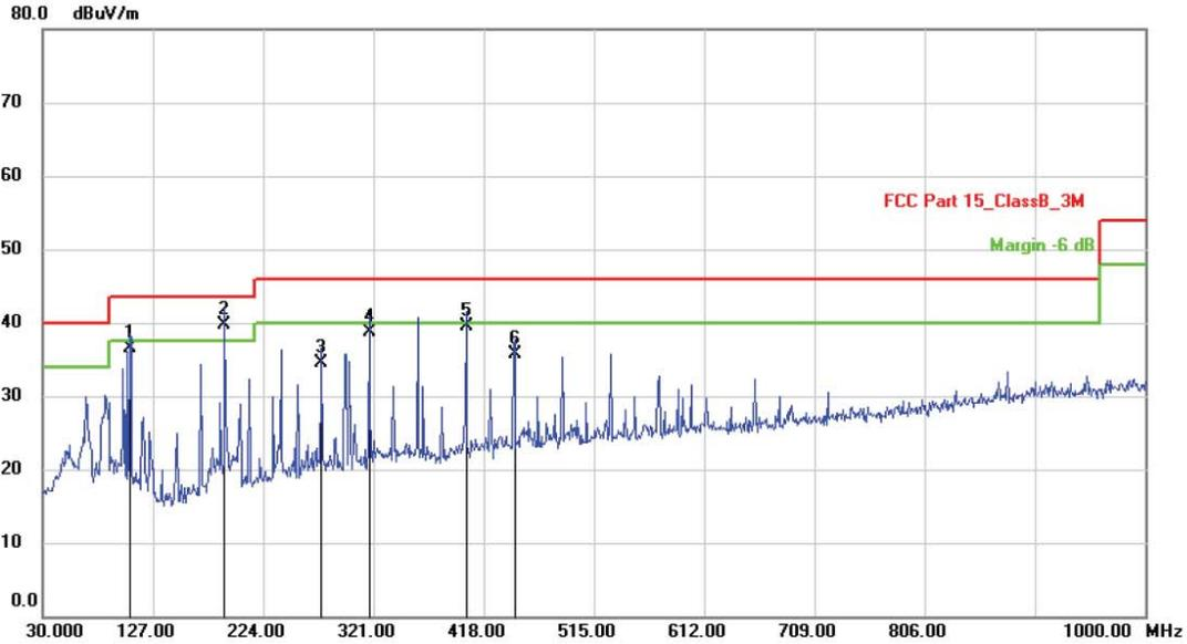
Site: 3m Chamber Polarization: *Horizontal* Temperature: 26
