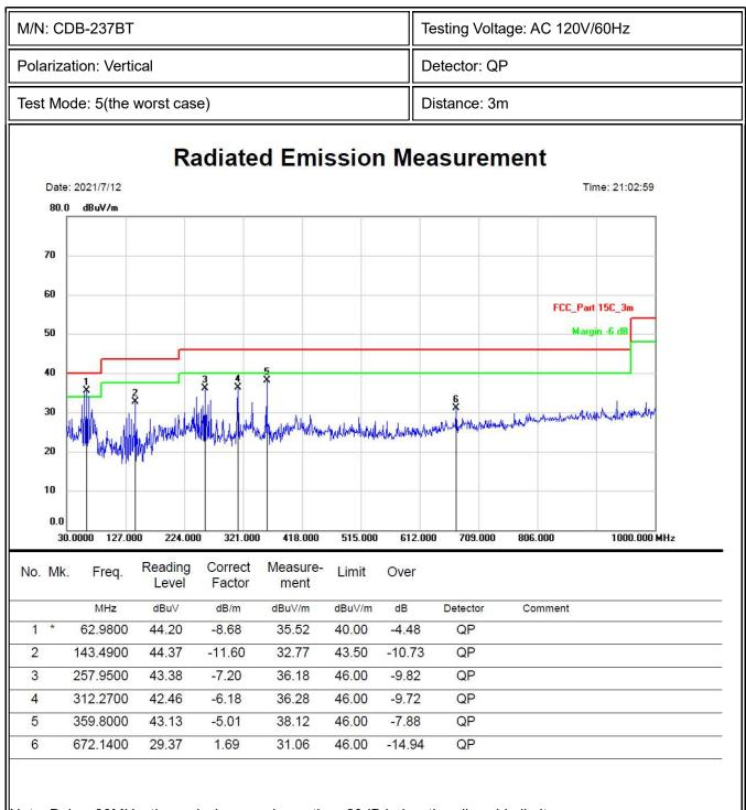
Note: Below 30MHz, the emissions are lower than 20dB below the allowable limit.
