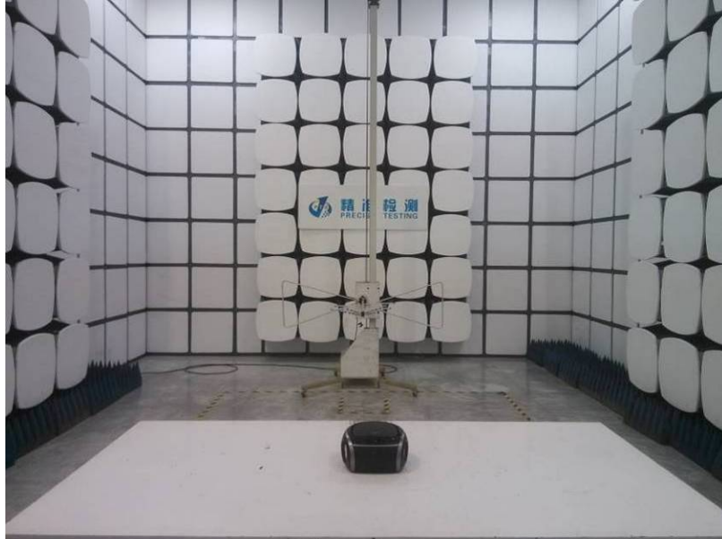
Radiated Spurious Emissions Test Frequency From 30MHz-1000MHz
