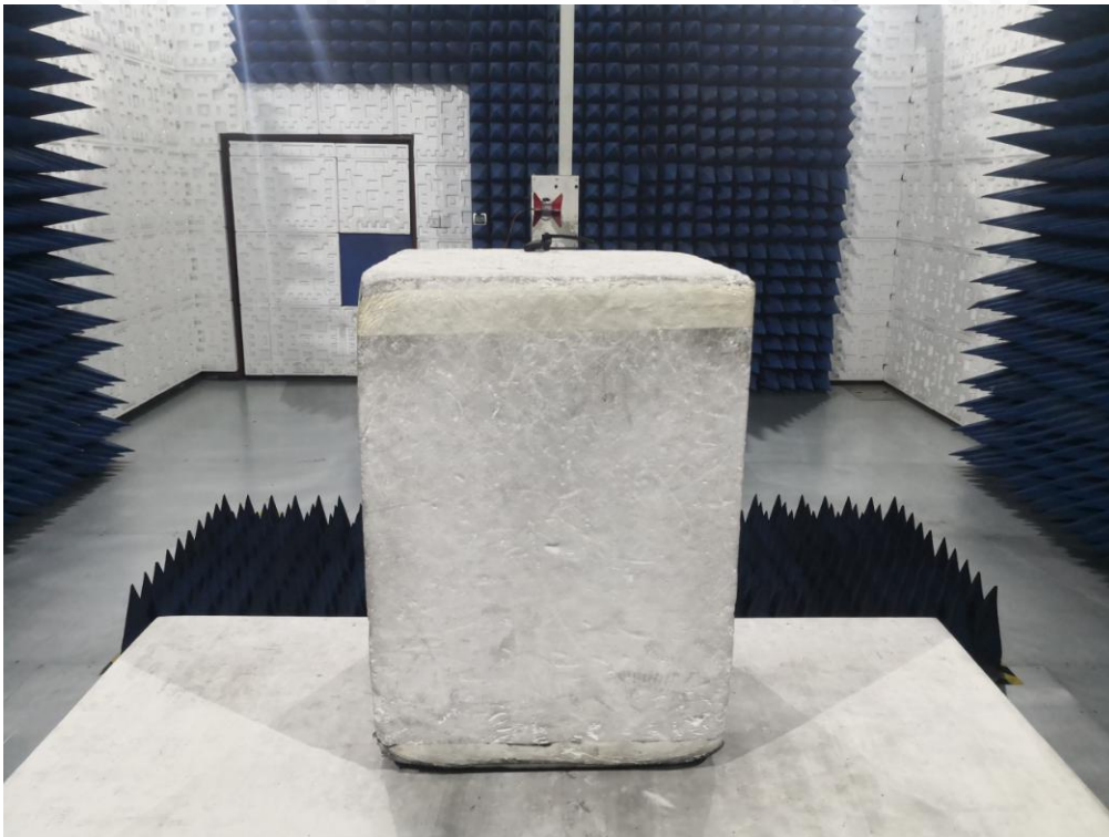
RADIATED EMISSION TEST SETUP ABOVE 1GHZ
