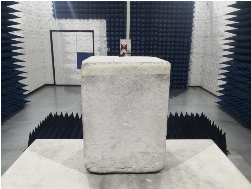
RADIATED EMISSION TEST SETUP ABOVE 1GHz
