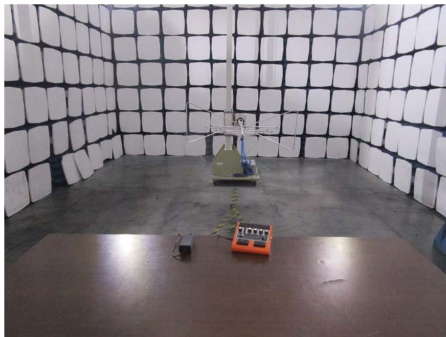
**Radiation Emission Test Setup (Above 1GHz)**
