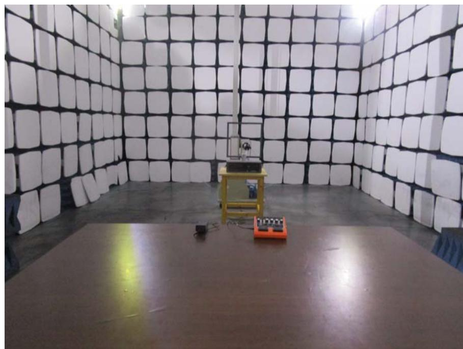
**Radiation Emission Test Setup (30MHz to 1GHz)**
