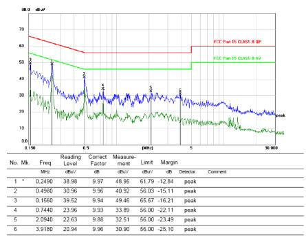
Note: Measurement=Reading Level+Correc Factor. Factor=(LISN or ISN or PLC or Current Probe)Factor+Cable
