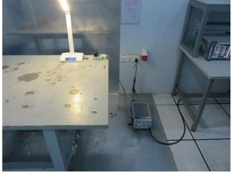
2. Photo of Radiation Emission Test
