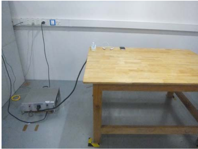
Conducted Emissions Test Setup – Front View
