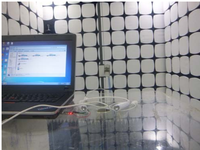
Radiated Spurious Emissions Test Above 1GHz
