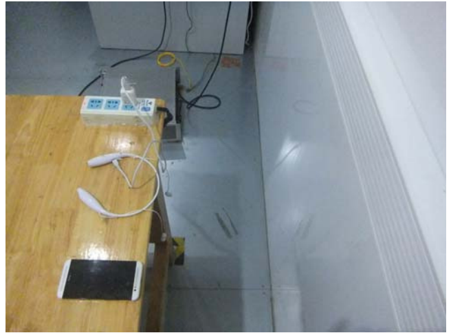
Conducted Emissions Test Setup – Side View
