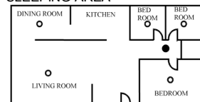
Figure 1: LOCATIONS FOR PLACING SMOKE ALARMS FOR SINGLE RESIDENCE WITH ONLY ONE SLEEPING AREA
