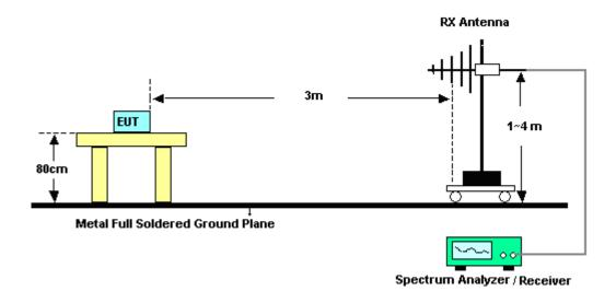
For radiated test from 1GHz to 18GHz
