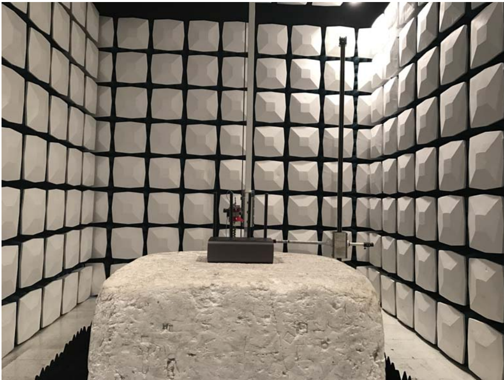
Description: Radiated Emission Test Setup for 1~18GHz
