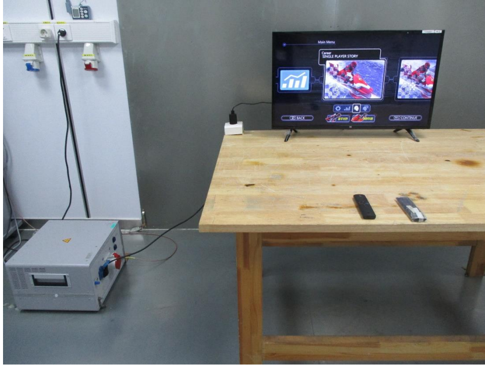
Conducted Disturbance Emissions on AC mains
