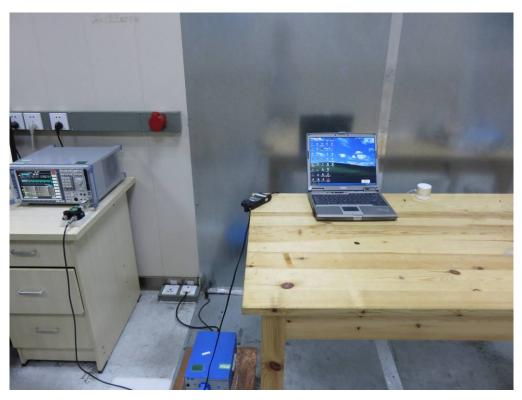
FCC RADIATED EMISSION TEST SETUP
